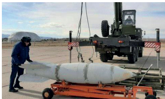
(All rights reserved) An IAB-500 dummy bomb used to simulate a gravity-operated nuclear munition, such as those carried on Su-24M and Su-34 bombers.
