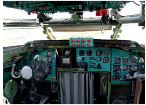
(PG) Without state-of-the-art multifunction touchscreens: the cockpit of an unmodernised Tu-95MS strategic bomber.
