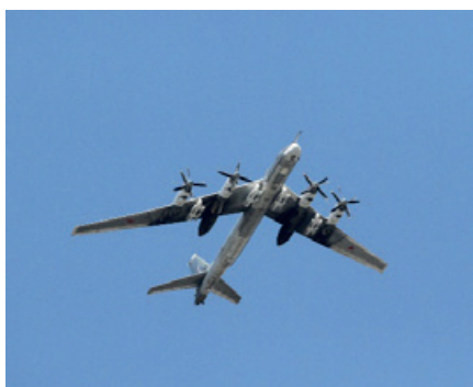
(PG) The four light grey pylons under the wing of this Tu-95MS indicate the carrying capacity of the Kh-101 missile.
