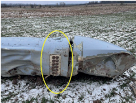
(All rights reserved) On 26 January 2023, circled in yellow is the L-504 decoy launcher, which has been newly observed on a Kh-101 cruise missile.
